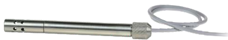
PPQ-621-XX-X-X Cable probe Ø12, L=200 mm, housing SS 316L, filter from SS mesh 25 µm
