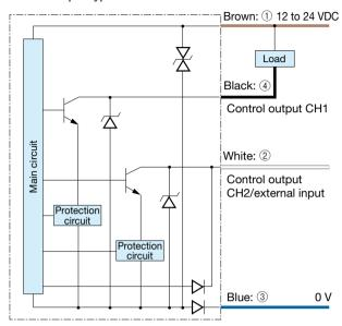
\*The D2□F-TS□□□ slave unit does not have power supply wires (brown/blue) because power is supplied from the master unit.
