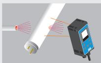
This is for the inspection process of a fluorescent light. By using a backlight and rotating the fluorescent tube the CVS1 EASY is able to identify a small pinhole.
